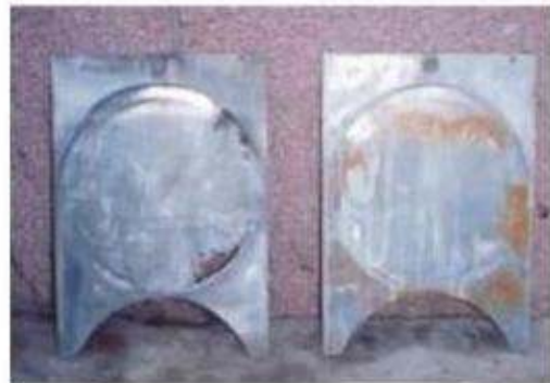
Stainless steel wedge gate disc after 1 week in service
