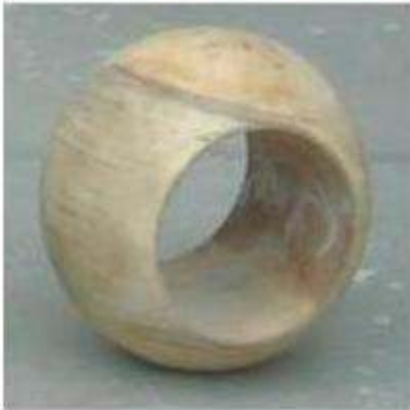
SK ceramic ball after 2 years in service in the petrochemical industry
