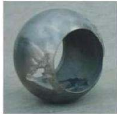
Metal ball after 1 month of use in the petrochemical industry
