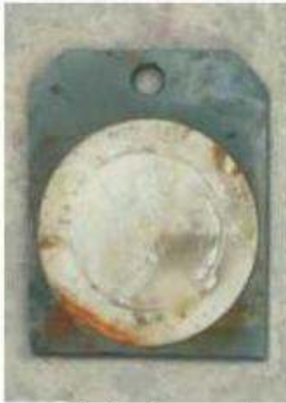
SK wear resistant ceramic wedge gate disc after 5 years in operation
